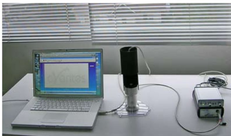
Portable UV-Vis spectrometer developed by SSEF Swiss Gemmological Institute in collaboration with the Physics Department of the University Basel. The instrument uses a small spectrometer, which just has to be plugged into a laptop (see last page!). © M.S. Krzemnicki, SSEF 2008
