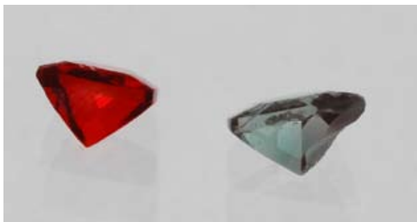
Red and green labradorite analysed with LA-ICP-MS to gain insight in the copper concentration of these feldspars. © M.S. Krzemnicki, SSEF 2008
